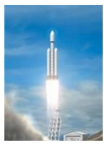
The Falcon Heavy could put 117,000 pounds into the same orbit as the International Space Station. The space shuttle hauls about 54,000 pounds into orbit. The old Saturn V could carry more than 400,000 pounds of cargo.
