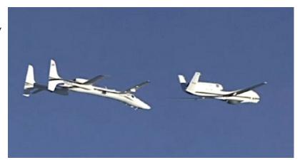
The lead receiver aircraft extended and retracted its aerial refueling hose several times, completing all planned tests to validate the associated program hardware and software.
