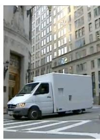
The vans, says Greenberg, "bounce a narrow stream of x-rays off and through nearby objects, and read which ones come back. Absorbed rays indicate dense material such as steel. Scattered rays indicate less-dense objects that can include explosives, drugs, or human bodies. That capability makes them powerful tools for security, law enforcement, and border control."
