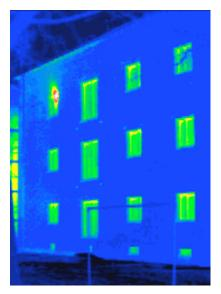
The website also explains the <u>benefits of thermal imaging</u>. According to Sagewell, the images provide far more information than a visual assessment would, including whether insulation is missing from a large part of a wall, sill, or foundation, or if there is a substantial heat leak from two single pane windows.
