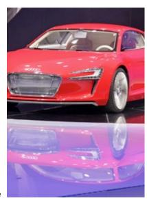
The Audi e-Tron is a fully electric vehicle with a driving range of 154 miles on a charge. It recharges in six to eight hours, so when you plug it in, you will have a "full tank," so to speak, by morning. It's definitely not for long hauls, however.
